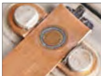
Weld copper sheet to copper electrode
