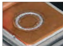
Weld Cu-Al composite sheet to aluminium electrode
